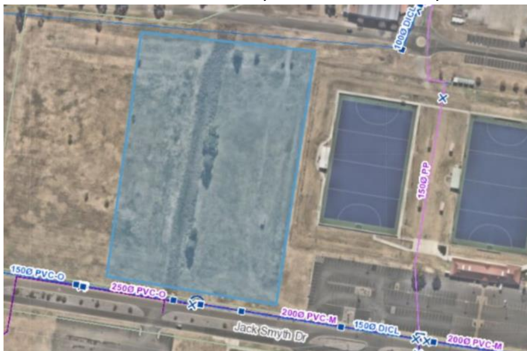
Figure 19 Tamworth Council Existing Water mains
