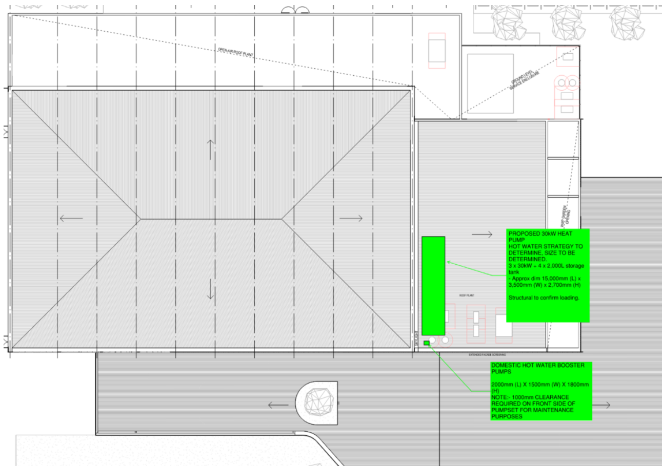
Figure 25 CO 2 Hot Water Heat Pumps & Storage Tanks Location
